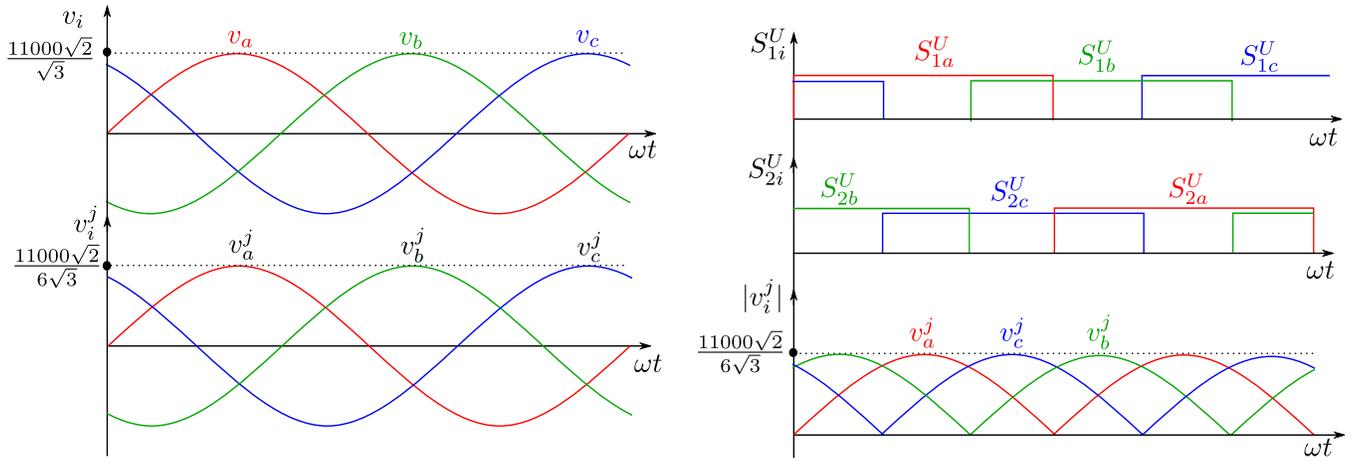
Fig. 3: Modulation of line frequency unfold
