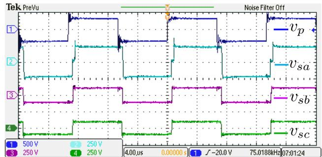
Fig. 11: HF transformer voltage waveforms in a module
