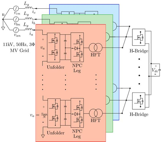
Fig. 1: Single stage MVAC to LVDC converter
