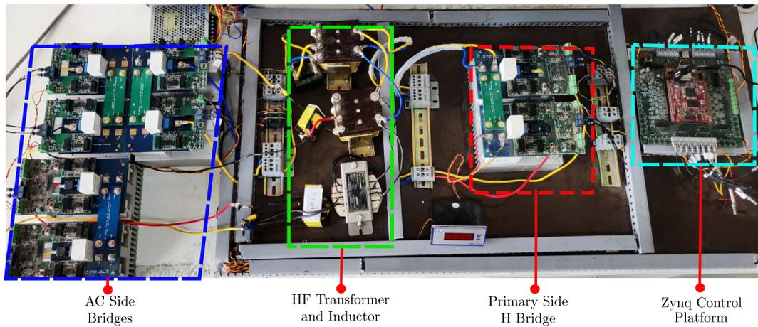
Fig. 7: Experimental Set-up
