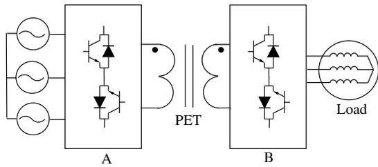
Fig. 1. Topology based on indirect modulation (A1)
