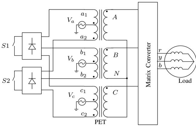
Fig. 3. Topology based on push-pull configuration (B1)
