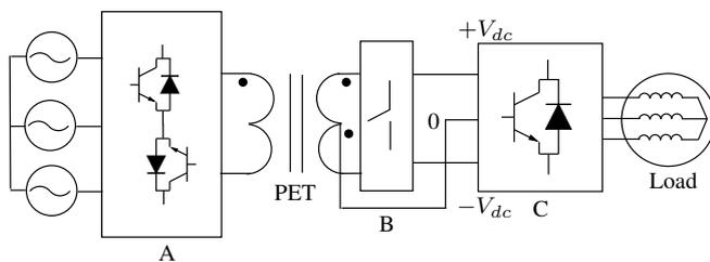
Fig. 2. Topology for common-mode voltage suppression (A2)
