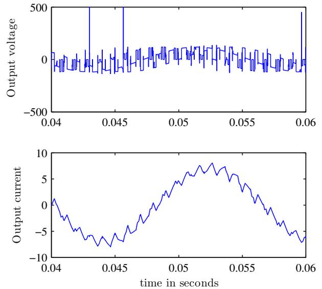
Fig. 14. Output voltage and current with source based commutation
