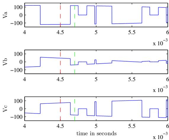
Fig. 7. Voltage across primary winding of transformer
