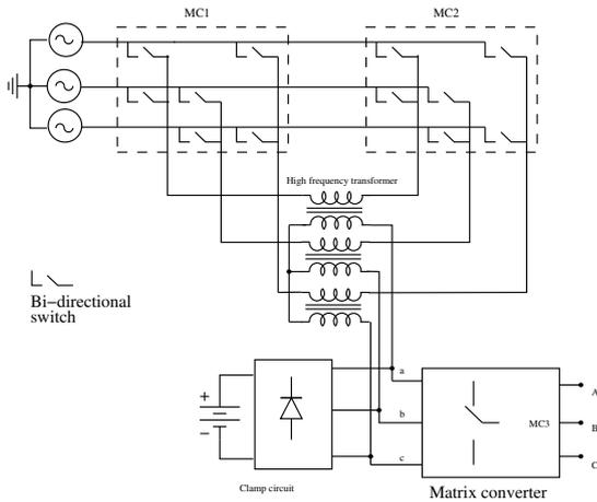
Fig. 1. Matrix converter driven high frequency transformer
