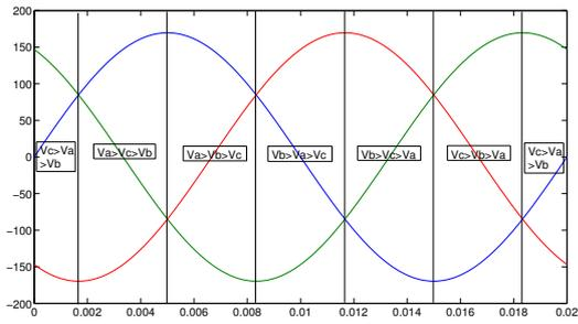
Fig. 5. Six voltage inequality conditions in three sine waves
