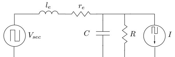
Fig. 3. Equivalent circuit of the transformer secondary
