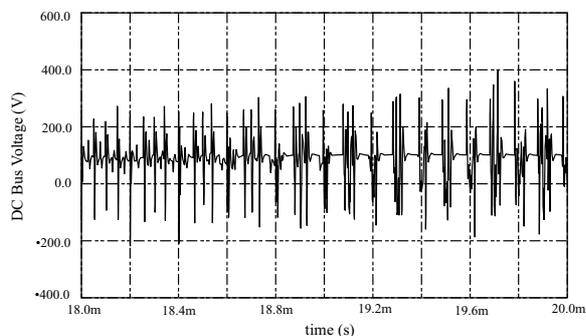
Fig. 9. Simulation result: positive DC link voltage
