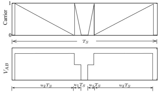
Fig. 5. Variable slope carrier and primary voltage over a subcycle
