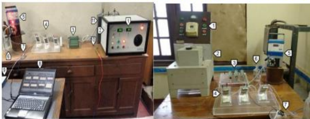
Fig.4. Experimental arrangement for AC/DC Inclined plane (10kV HVAC/DC)
