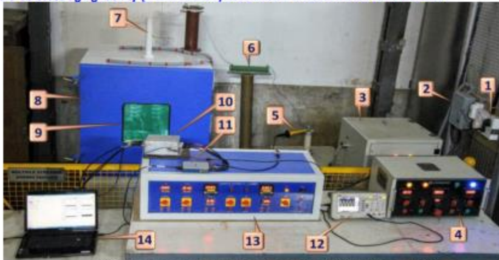
Fig.6 Developed Multi stress aging facility (30kV HVAC and DC)
