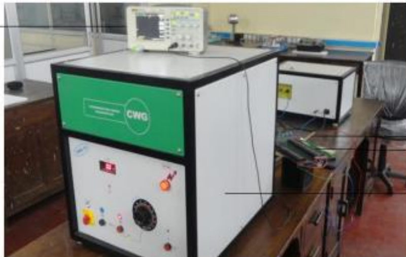
Fig. 9 Combination/hybrid wave generator (1.2/50 & 8/20 \mu S)
