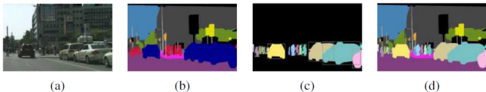
Figure 6.32 Examples of image segmentation (Kirillov, He et al. 2019) © 2019 IEEE: (a) original image; (b) semantic segmentation (per-pixel classification); (c) instance segmentation (delineate each object); (d) panoptic segmentation (label all things and stuff).
