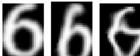
Figure 5.28 An original "6" digit from the MNIST database and two elastically distorted versions (Simard, Steinkraus, and Platt 2003) © 2003 IEEE.
